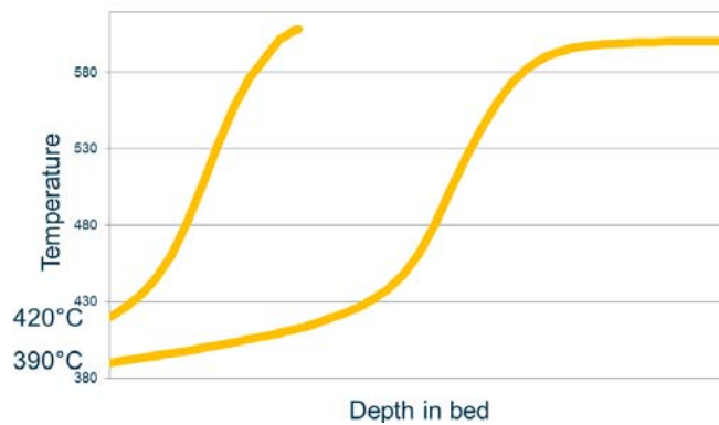
Figure 5: Effect of increasing the inlet temperature from 390°C to 420°C on the temperature profile
